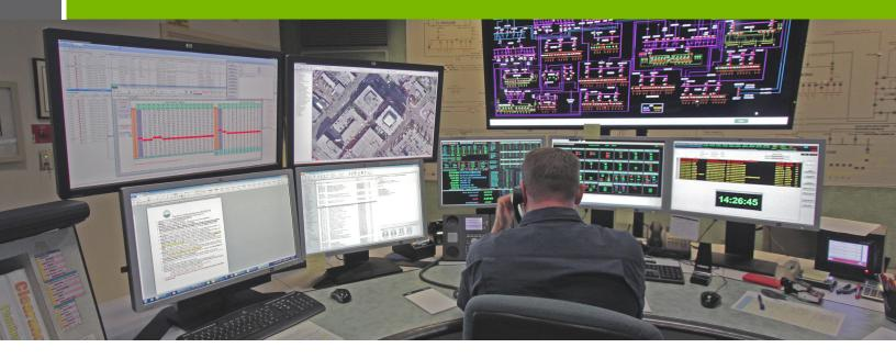
Landis+Gyr's Transmission and Distribution SCADA software (TDS) simplifies the management of both large and small utility control centers. The solution is a distributed client/server SCADA system that supports multiple front-end processors, servers, and operator workstations. It includes voice synthesis, areas of responsibility, automatic alarm inhibit, customizable alarm sounds, and other advanced functions.
