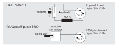
Characteristics of switch version according to DIN EN 50227 (Namur):
