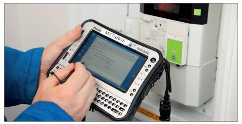
The Site Manager installation tool transfers work orders to installation personnel without manual work. It enables multiple functionality to include the wireless storage of meter data and meter time setting.
